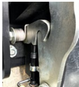
Automatic lock in up-right position
